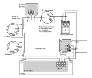
As every loop device has an isolator fitted, it is not necessary to apply special attention where there are more than 32 devices. However no more than a maximum of 512 input devices shall be installed on one control panel.
