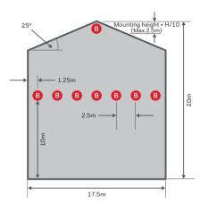
One beam detector covers 18.75m using extra % allowed due to angle of roof.
