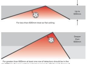
top 600mm. For apex ceilings extend coverage by 1% for each degree of angle up to a maximum of 25%
