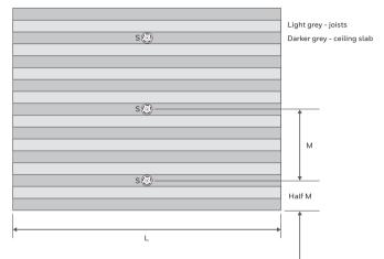
Permitted spacing is detailed in the table below: ratio between ceiling heights vs beam depth and maximum spacing 'M'.
